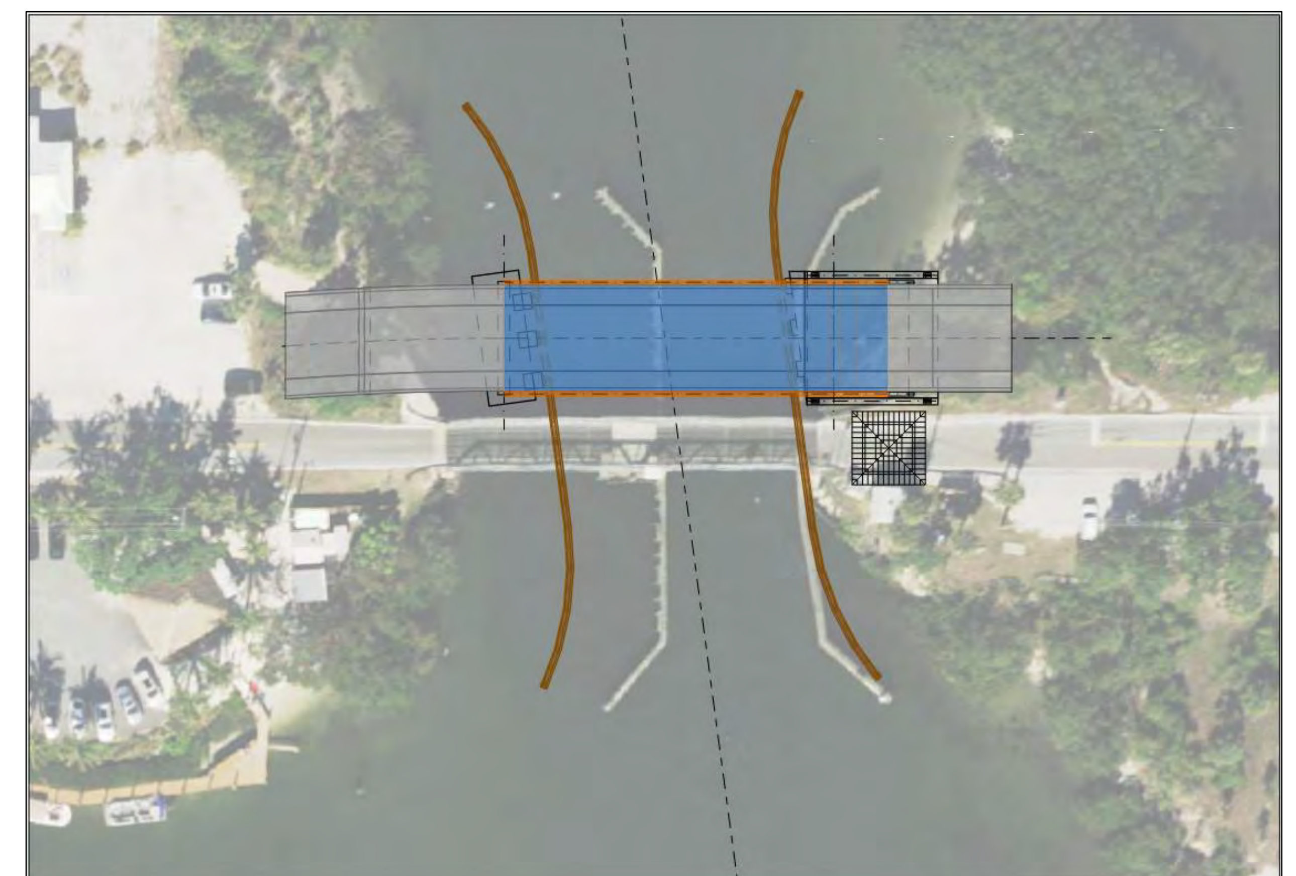
Bascule Bridge on Temporary Alignment to the North
