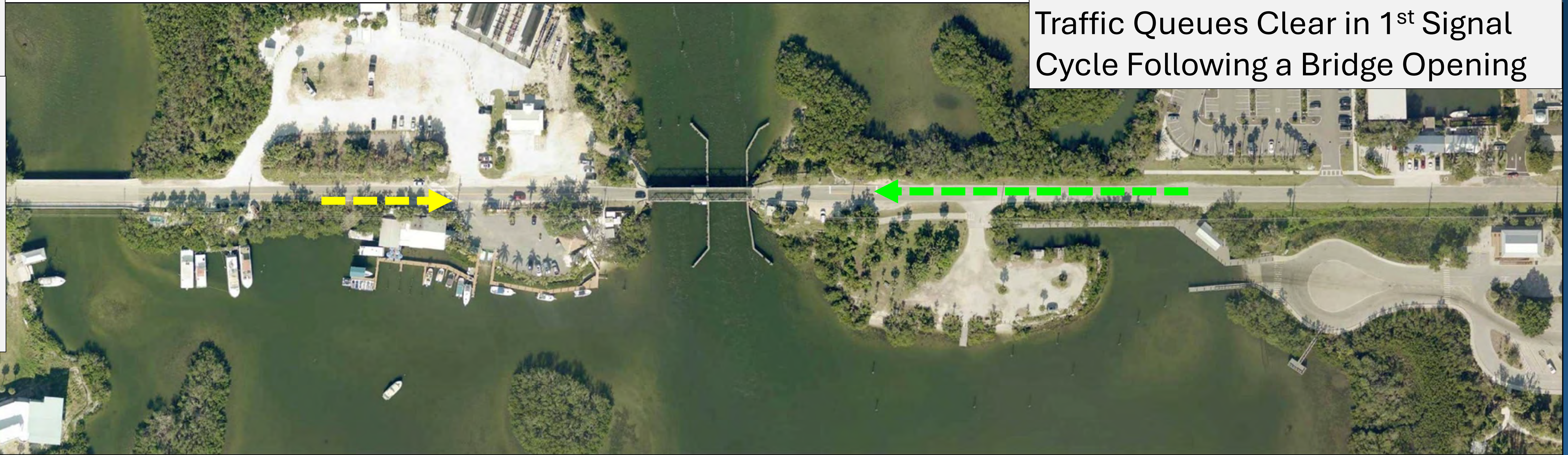
AM Peak Hour Traffic – Queue following a 7-minute Bridge Opening
