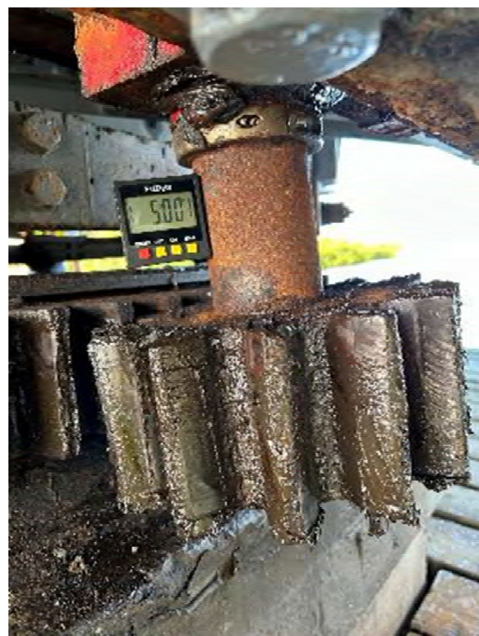
Bent Main Pinion Gear Shaft
