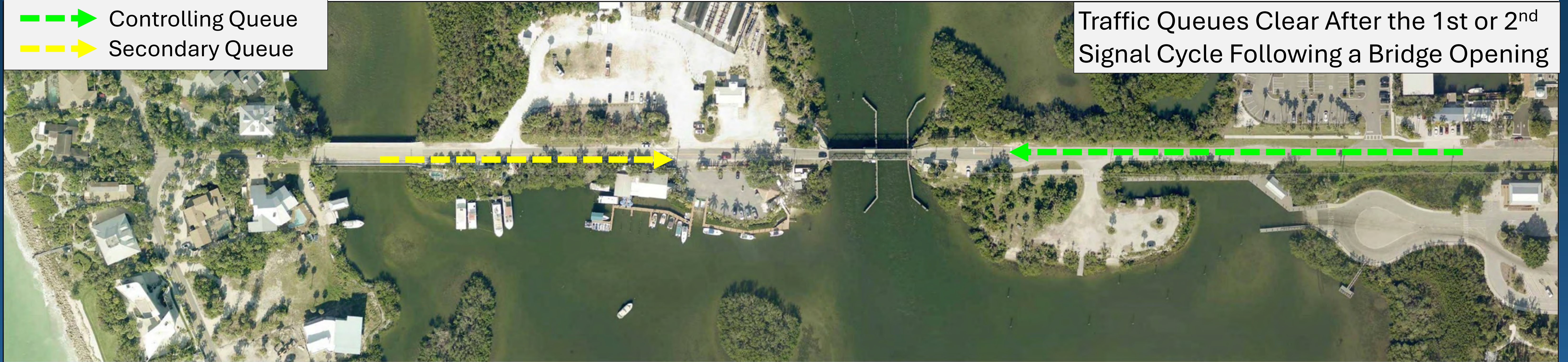
AM Peak Hour Traffic – Queue following a 7-minute Bridge Opening
