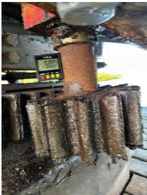
Bent Main Pinion Gear Shaft
